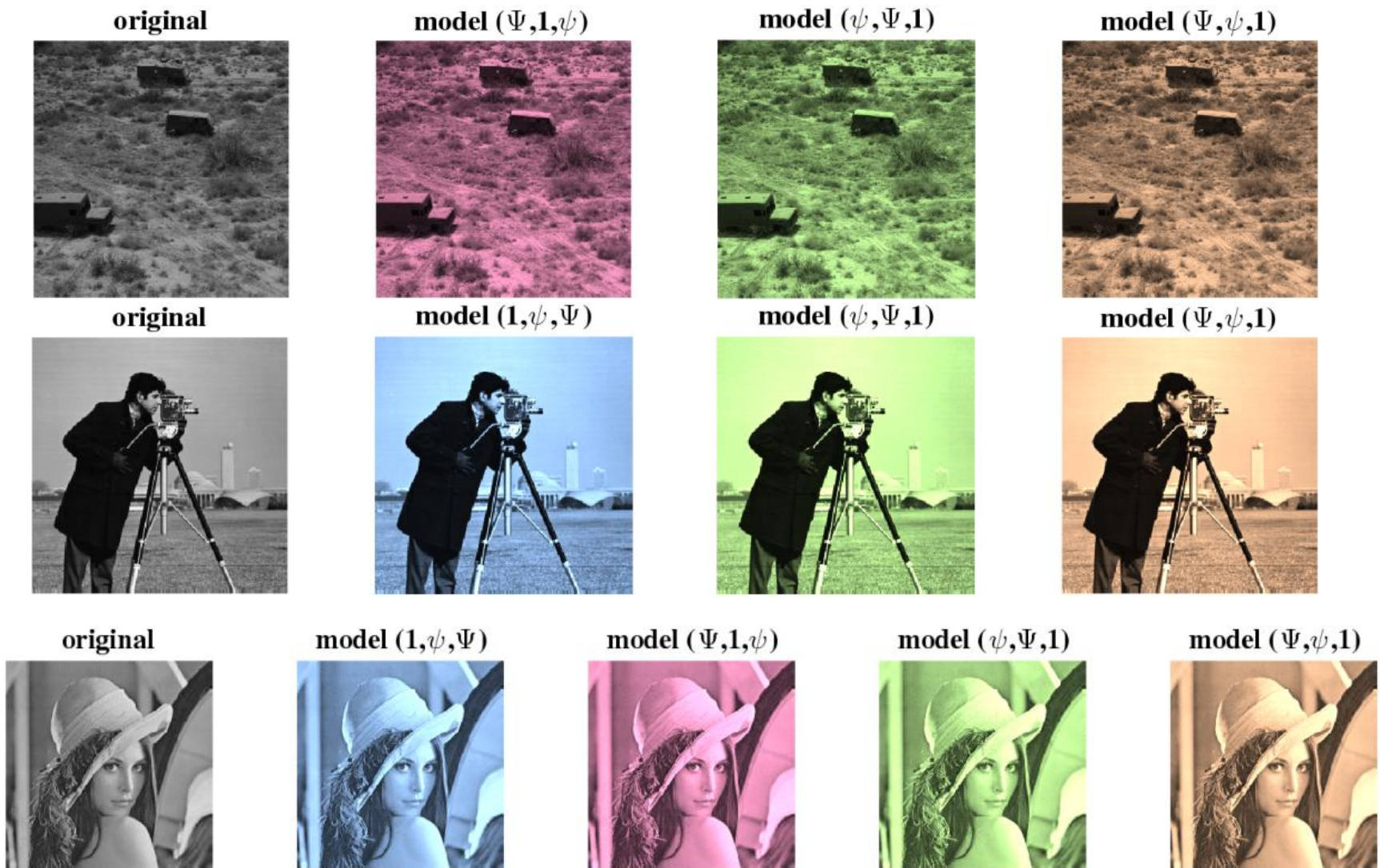
Figure 8. Grayscale images and the color images calculated in the (1, \sqrt{\Psi}, \Psi) , (\Psi, 1, \sqrt{\Psi}) , (\sqrt{\Psi}, \Psi, 1) , and (\Psi, \sqrt{\Psi}, 1) -models.
