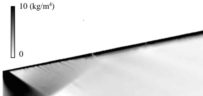
**Figure 5: Density Gradient of Throat Area Updated Contour**
