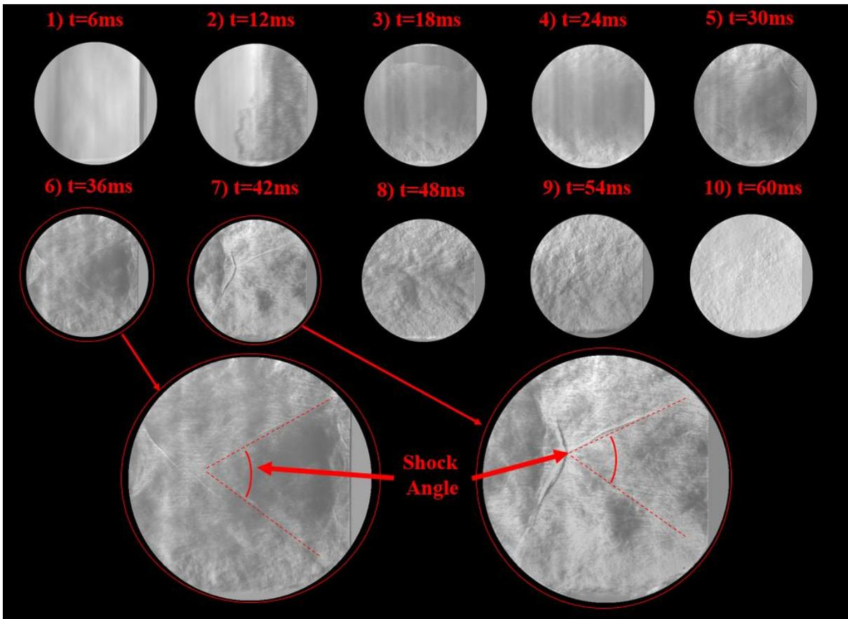
**Fig. 13: Schlieren Imaging for 3105-Aluminum Diaphragm Blow-out with 0.01-inch Remaining Thickness**
