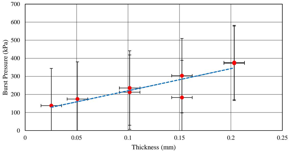
**Fig. 7: Aluminum Foil Thickness vs Burst Pressure**
