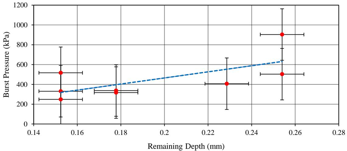
**Fig. 9: 3105-Aluminum Remaining Thickness vs Burst pressure**
