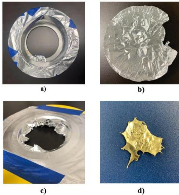
**Fig. 8: Post Rupture Aluminum Foil a) & b) 1 Layer Fragmentation c) & d) 8 Layer Fragmentation**
