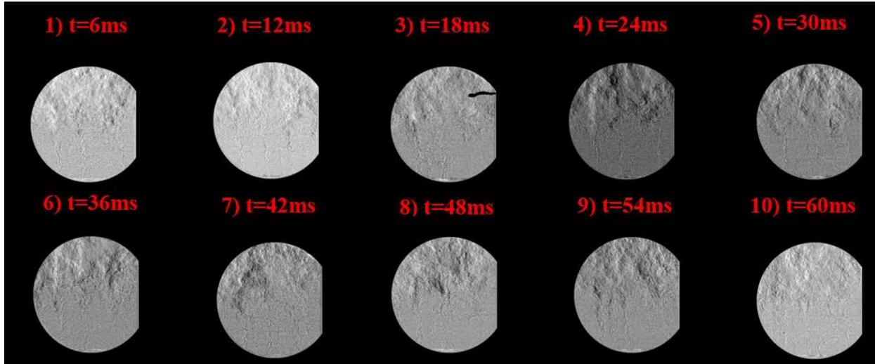
**Fig. 11: Schlieren Imaging for Aluminum Foil with 6 Layers**
