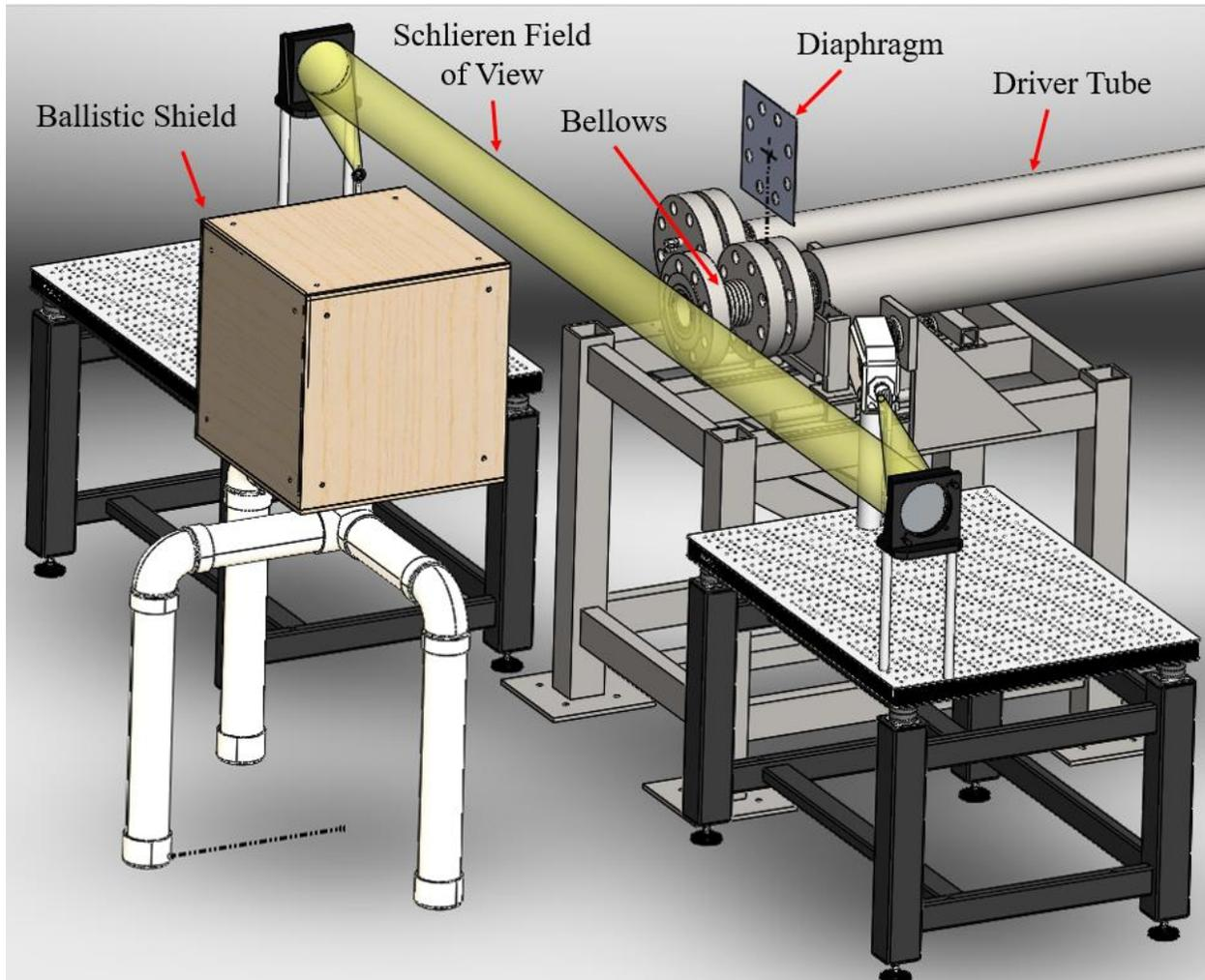
Fig. 6: Experimental Set-Up
