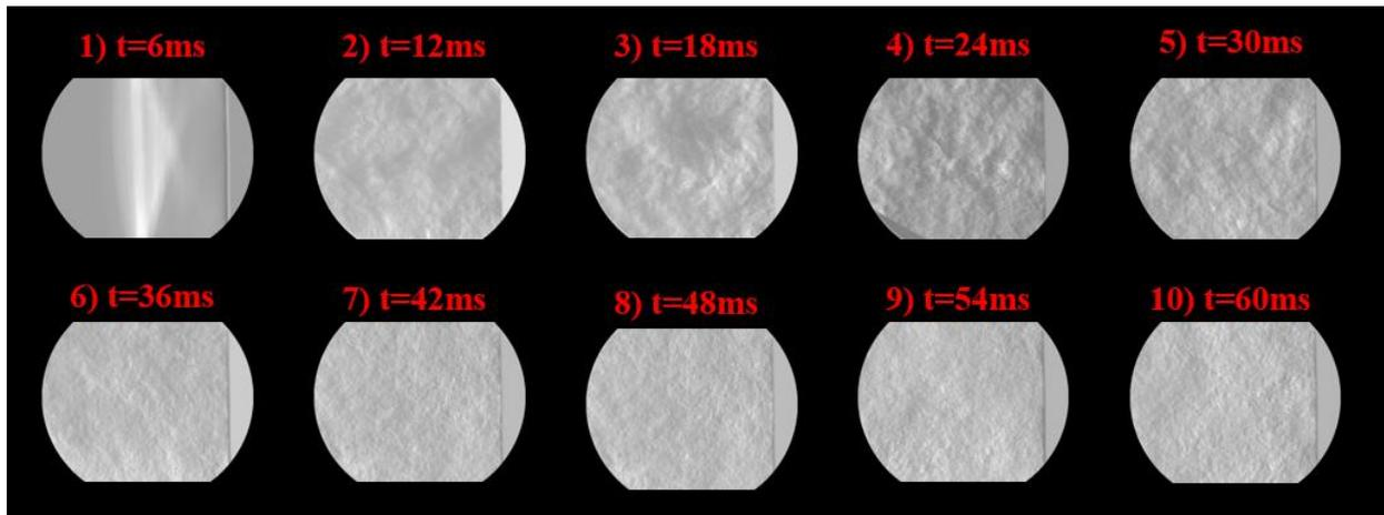
**Fig. 12: Schlieren Imaging for 3105-Aluminum Diaphragm with 0.009-inch Remaining Thickness**
