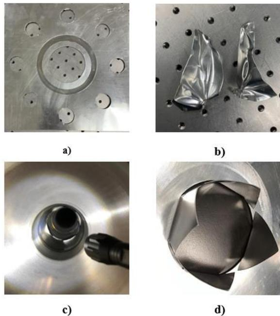
**Fig. 10: Post Rupture of 3105-Aluminum a) Fragmented Rupture b) Fully Petaled**
