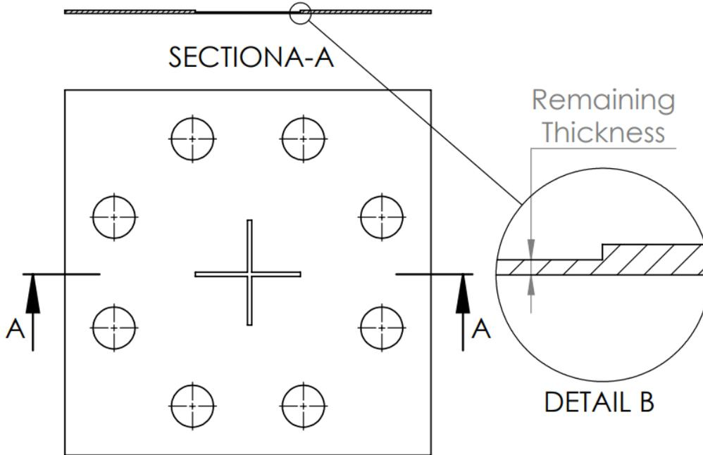
**Fig. 3: Reference for Remaining Thickness**
