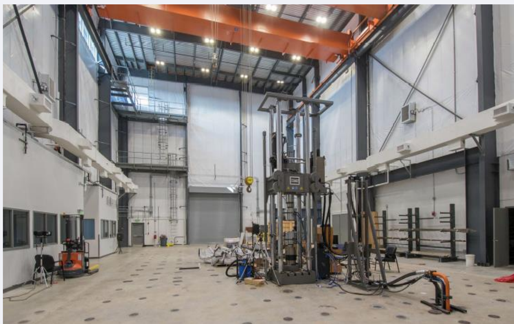
Fig. 3 LST Lab Interior and Visual of the Floor Anchor Points
