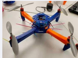
Fig. 2 Final look of the drone with 3D printed parts, R pi, designed circuit board, and power supply
