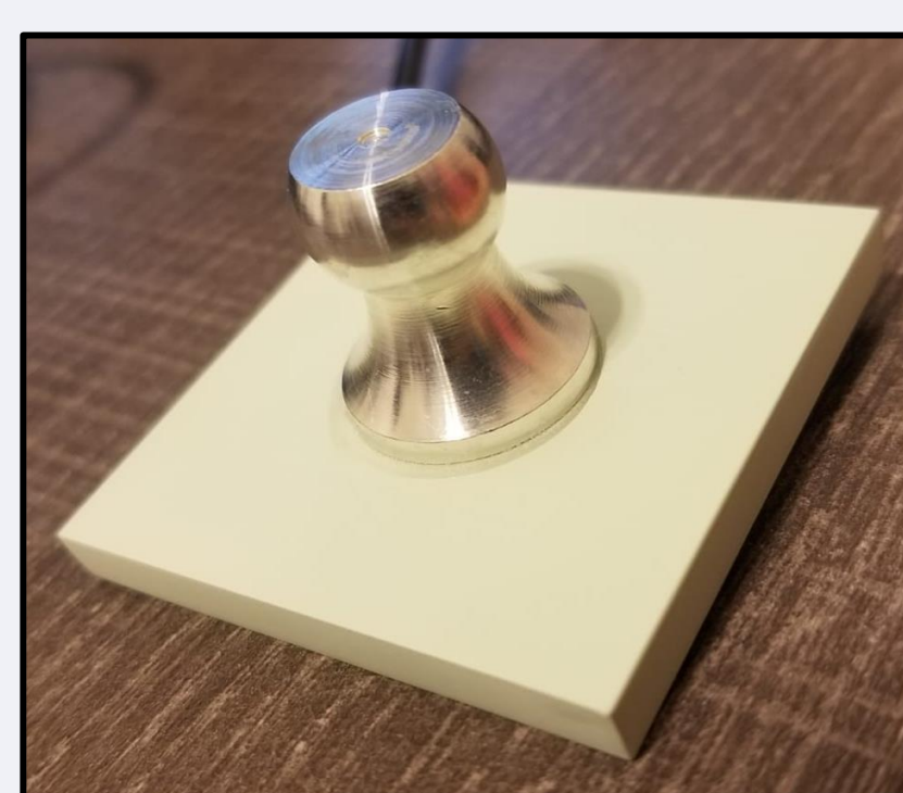
Fig. 3 Sample with Adhered dolly for pull-off test following ASTM D4541.
