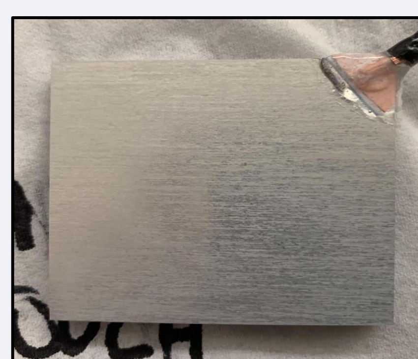
Fig. 2 Sample after the anodization process
