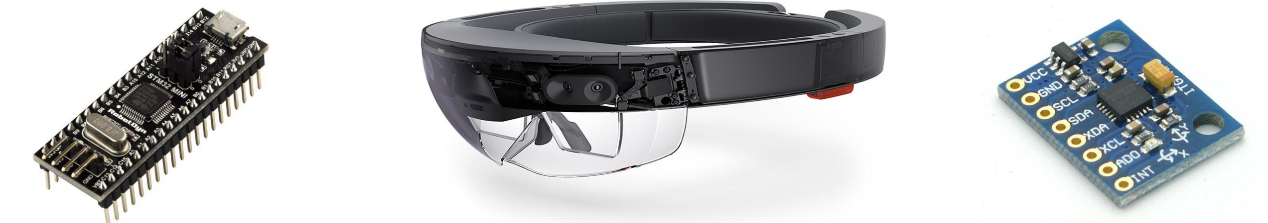
Figure 3. Hardware as seen from left to right: ESP32 Microcontroller, Microsoft HoloLens 2, and IMU MPU 6050
